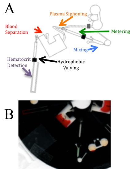
**Figure 1:** (A) CorelDRAW design of protein colorimetric analysis PeT LPMD. Each function of the design is designated by a colored arrow. (B) Photograph of a LPMD after analysis.
