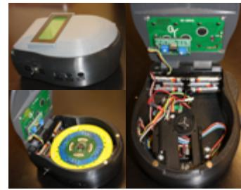
**Figure 2:** Rotational control system in 3D printed case.
