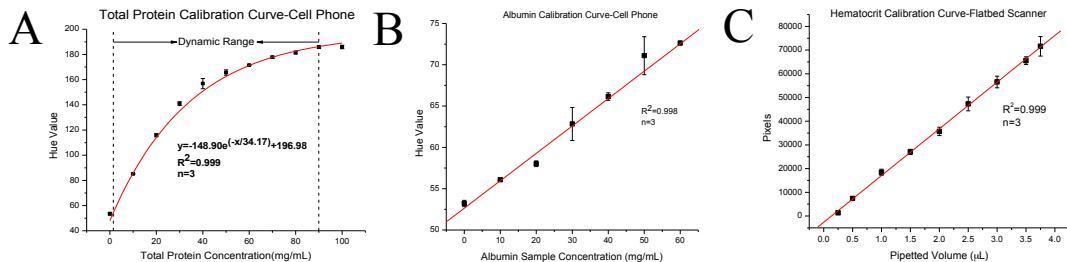
**Figure 3:** (A) Total protein calibration curve by cell phone detection and analysis. (B) Albumin calibration curve by cell phone detection and analysis. (C) Hematocrit calibration curve by flatbed scanner and Wolfram Mathematica 8 image algorithm.
