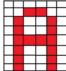
Fig. 4. The letter A is represented by the pixel sequence 000000001100010010010010010011110010010010010010010
