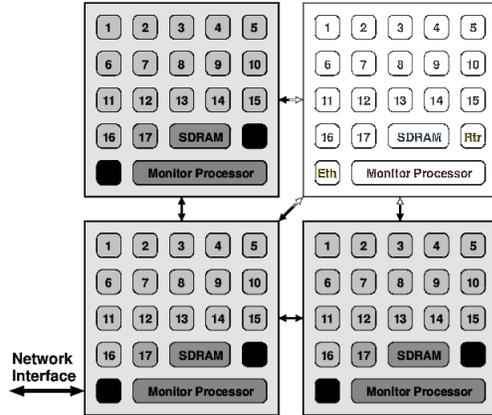
Fig. 5. Illustration of three input and one output chips on the SpiNNaker machine. The input chips consist of 9 total inhibitory neurons and 39 total excitatory neurons. Each of the output neurons are excitatory.
