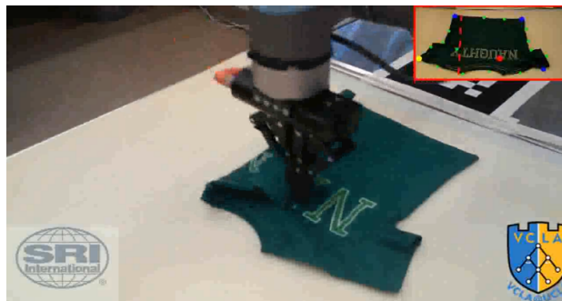
Figure 1: The robot autonomously performs a cloth folding task after learning from a human demonstration.
